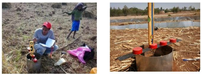
Picture S1: Measuring pre treatment left and post treatment right steady state infiltration rate
