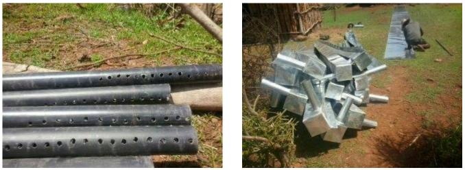
Picture S3: Perforated pipe for ground water recharge monitoring (left) and collector channel to drain event runoff from plots to runoff tank (right)
