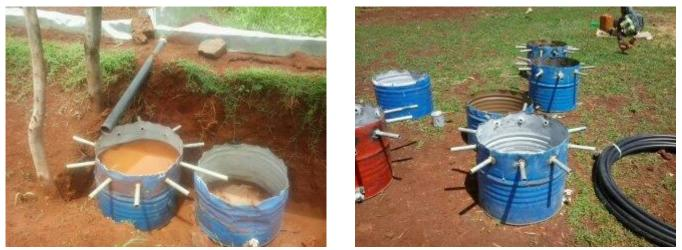
**Picture S6: Tank for runoff collection (runoff barrel)**
