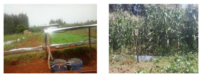
Figure 3.4: Runoff barrels (left) and manual rain gauge (right) installed to collect surface runoff and daily rainfall respectively
